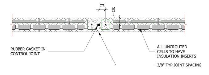
NOTE: ALTERNATE STANDARD HALF CMU WITH OMNI JAMB BLOCK AT CONTROL JOINT SAW CUT NOTCH IN OMNI JAMB BLOCK TO ACCOMMODATE RUBBER GASKET
