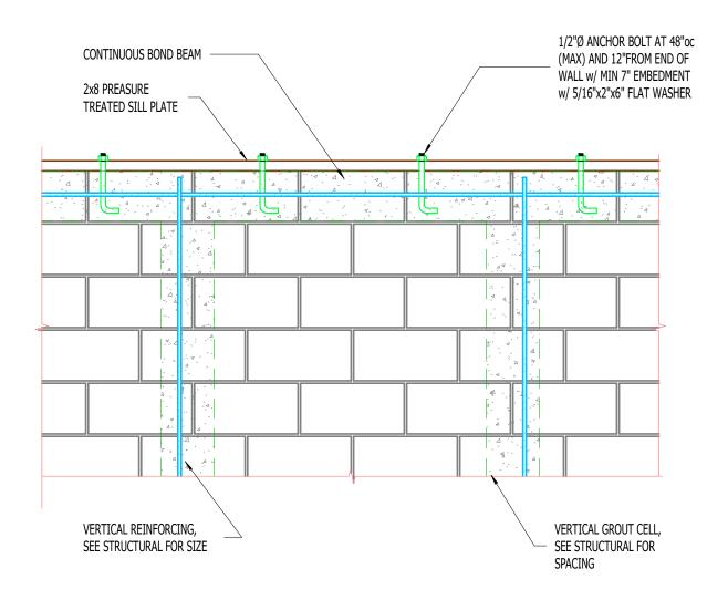
7 WALL TO ROOF SILL PLATE (ELEVATION)
