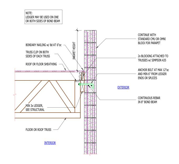
LOAD BEARING LEDGER w/ TRUSS TOP CHORD SUPPORT
